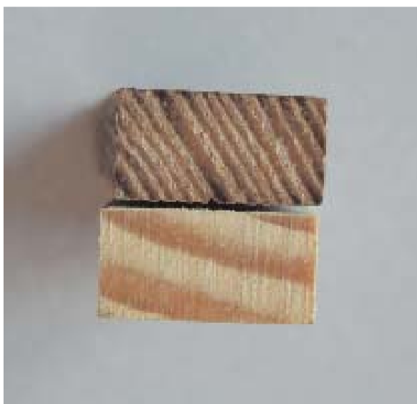
The cross grain of the old-growth pine used for most historic windows (above) is very dense, helping to create a very durable wood. This old pine has a much longer life-span than either the new-growth pine (below) or vinyl used in most replacement windows.
